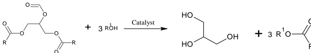
**Equation 1:** General equation for biodiesel synthesis from vegetable oil via transesterification.
